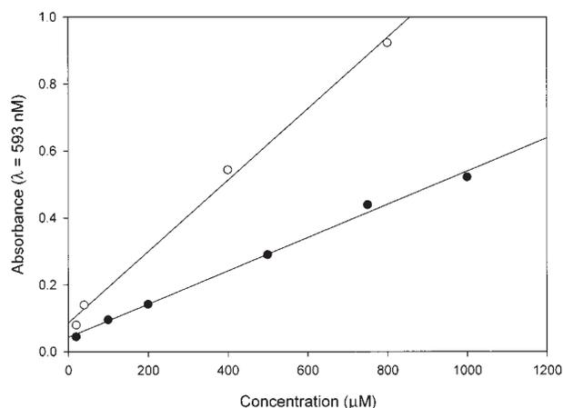
**Fig. 1.** Results for the FRAP assay for 5-ASA in solution. The response curve for 5-ASA (open circle) ( $R^2 = 0.9954$ ) and for standard Fe(II) (filled circle) ( $R^2 = 0.9949$ ). The activity of the antioxidant was determined from the slope ratios of 5-ASA and Fe(II) to be 2.21, indicating the antioxidant capacity of the compound. Each point represents the average of 4 measurements.
